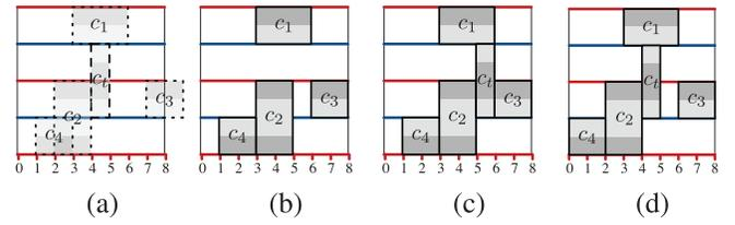
Fig. 3. Comparison between MLL and our proposed MGL. (a) GP. (b) Four cells legalized; Final results of minimizing the total displacement w.r.t. (c) current locations (MLL) and (d) GP locations (MGL).
